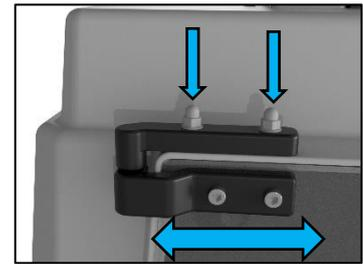
Loosen the top hinge/cabinet fixing. Move it so that the door becomes level in the frame and opens/closes freely. Tighten the fixings.
