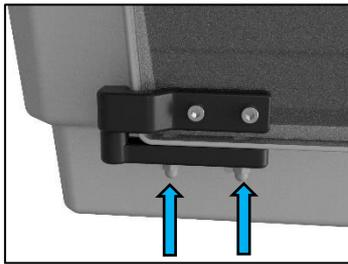
Loosen the bottom hinge/cabinet fixings by half a turn so that the hinge becomes free to move.
