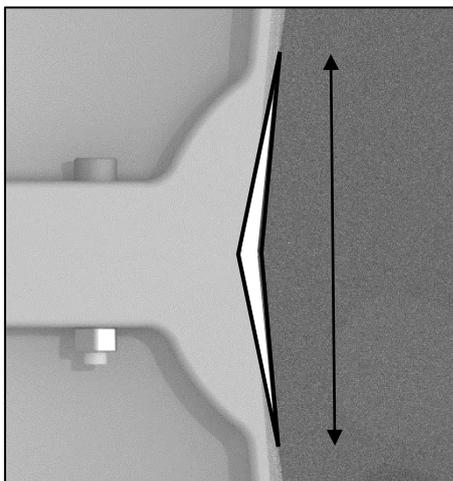
Observe the length of any 'V' shape gap that a claw could fit through. Cut the door edge strip to fill the length of the gap.
