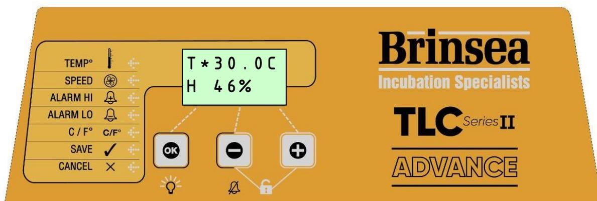
The TLC Advance Series II control system utilises highly accurate, individually calibrated sensors for temperature and humidity. Be cautious of low-cost analogue or digital thermometers and hygrometers when comparing them with the brooder/ICU display readings.
