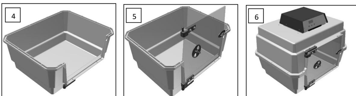
Fit the M4 x 30mm cap-headed screws, star washers and nuts into each set of holes around the edge of the cabinet. Tighten enough to prevent them spinning. This creates an air tight seal around the cabinet. If the nebuliser is required, fit the nebuliser bracket as shown (8a). If the nebuliser is not required fit the grommet first and secure it with the bracket (8b).
