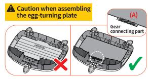
If the egg-turning plate is not assembled correctly, it may cause incubator failure. The gear connecting part(A)of egg-turning plate must be on the top side.
