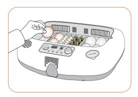
Mhen using the universal tray, there must be some gaps (approximately 2 mm) between the ABS divider and the egg for easy egg turning.
