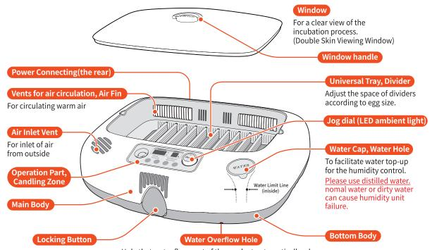
Hole that water flows out of the product automatically when you pour water into the water hole more than required amount (800cc).
