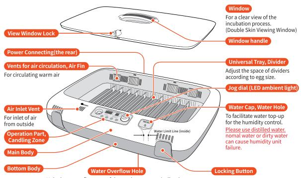
Hole that water flows out of the product automatically when you pour water into the water hole more than required amount(1400cc).
