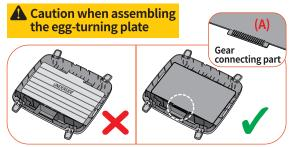
If the egg-turning plate is not assembled correctly, it may cause incubator failure. The gear connecting part(A)of egg-turning plate must be on the top side.
