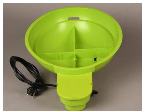
At the early stage just fill the first sector, after one hour check the humidity reading on the display, if it is low, then proceed to fill the 2nd sector and repeat the operation until the correct humidity of 47-50% RH is reached during the incubation phase; manage to grow up to 60-65% RH humidity the last 2 days during hatching phase.
