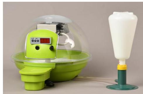
4. The base of the incubator consists of four sectors with different levels, by screwing or unscrewing the tank you will get an automatic filling of the different tanks. The four notches will indicate the water filling of the different tanks:
