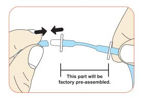
Please note that pumping performance will be reduced if the silicone tube isn't fitted tightly onto the nipple, or if the tube length is different from [Picture A].
